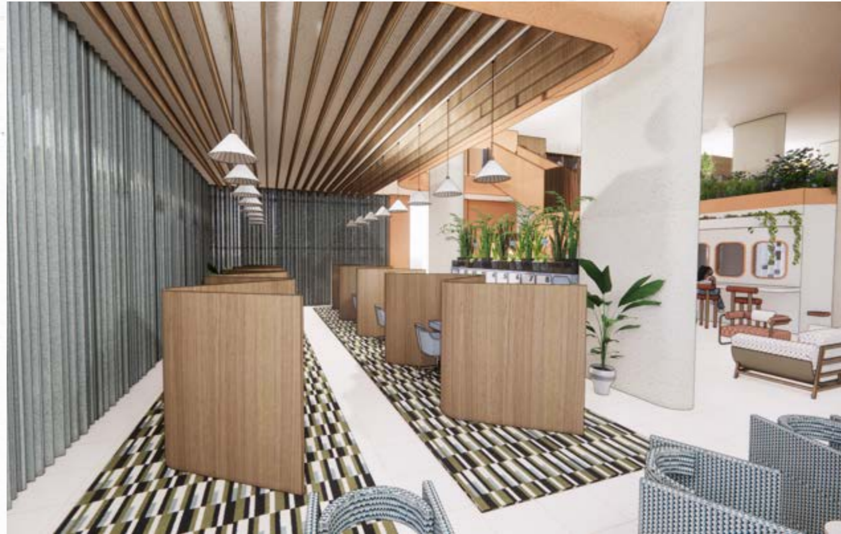
▲ QUIET CO WORKING PODS WITH BAFFLE CEILING FOR ACOUSITC PROPERTIES
