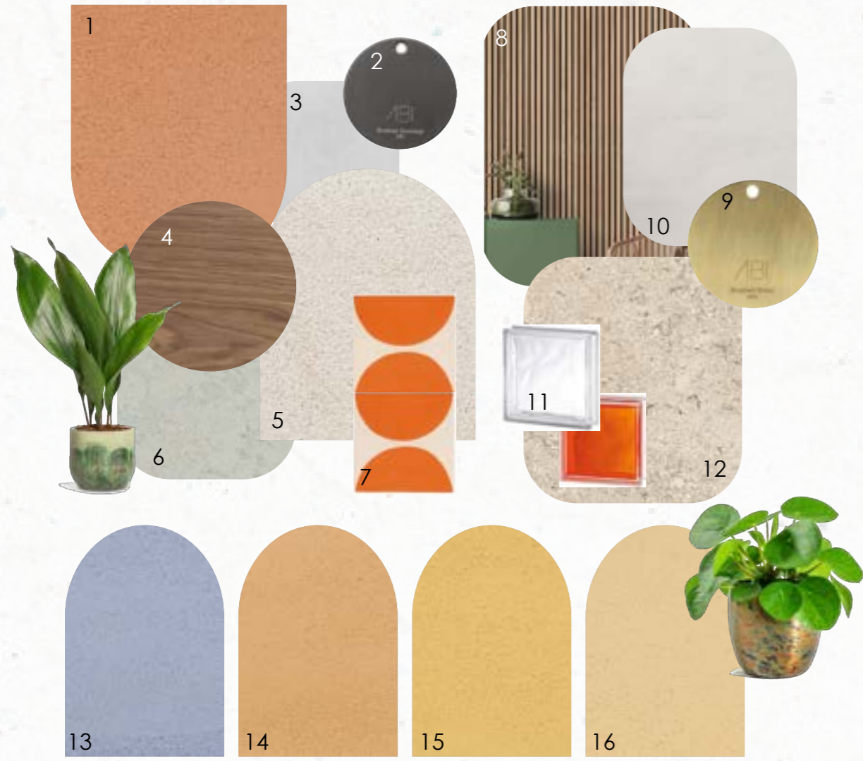
1. Clayworks Plaster, 2. Brushed Gunmetal, 3. Microcement, 4. FSC Certified Walnut Veneer, 5. Clayworks Plaster, 6. Forbo Marmoleum Flooring, 7. Recycled Tile 8. FSC Certified American Oak Batens, 9. Brushed Brass, 10. Quartz, 11. Glass Block, 12. Limestone Tile, 13-16. Clayworks Plaster
