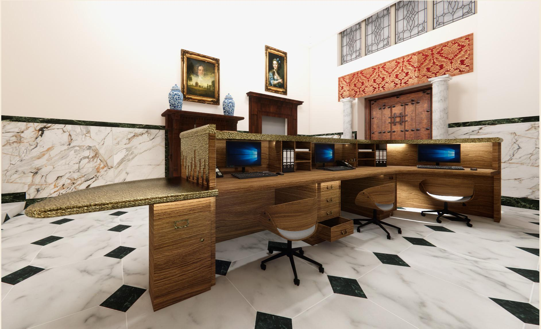
The interior of the desk showcases the **maximisation of desk space** to promote work flow. Space for three computers as well as ample storage has been offered, including filing shelves built to the specifications of the client's lever arch files. LED lighting has been used to illuminate the space. The lowered end blends seamlessly with the main body of the desk, allowing for **wheelchair access**.
