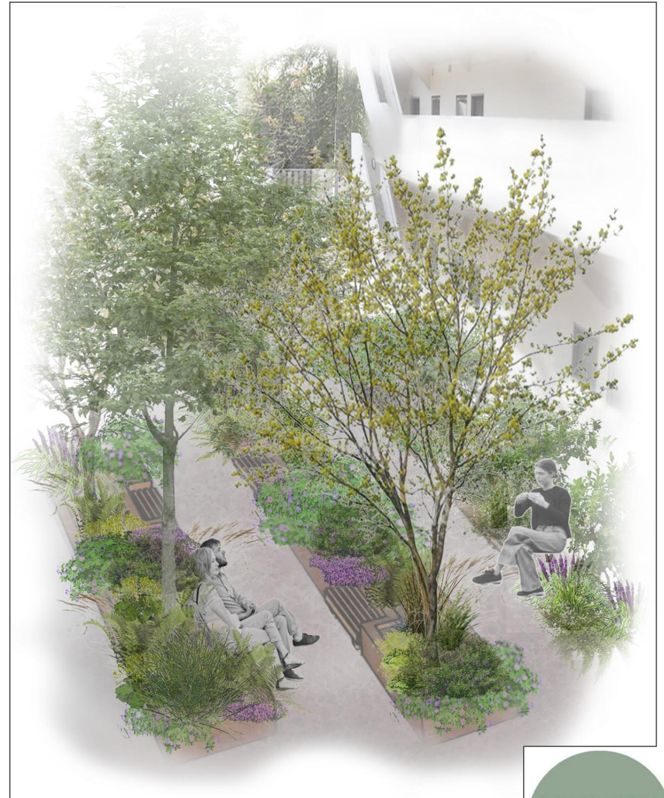
Concept visual of front of Isokon, modelled in SketchUp and rendered in Photoshop. The long raised planted beds with recessed seating are designed to accentuate and compliment the walkways at the front of the building.
