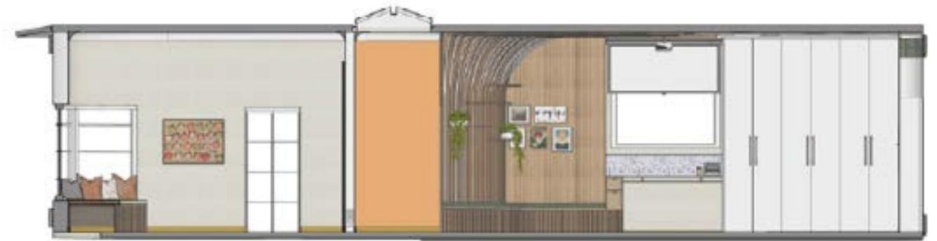
INTERIOR - Elevation showing from R-L, storage, window and work bench, curved structure and bench seating, bookcase and garden room with door to garden - not to scale
