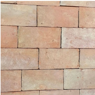
Bespoke pavers formed from brick rubble on site
