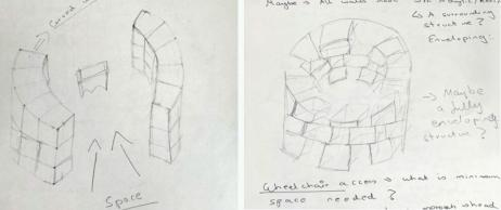
Chosen shape: Circular structure made from square resin blocks feeling of being surrounded, Contrast of squares and circles, Gaps between blocks can be used as entrances
